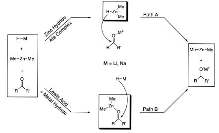
Figure 2. Possible mechanism for reduction of carbonyl compounds with metal hydride-Me<sub>2</sub>Zn reducing system.
